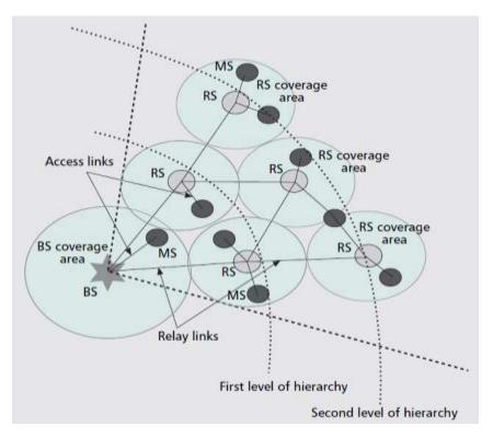
Figure 1: Base station with relay stations
